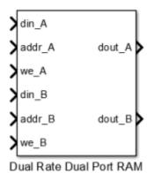
For more information about the block, see Dual Rate Dual Port RAM. For HDL code generation details, see Dual Rate Dual Port RAM.
